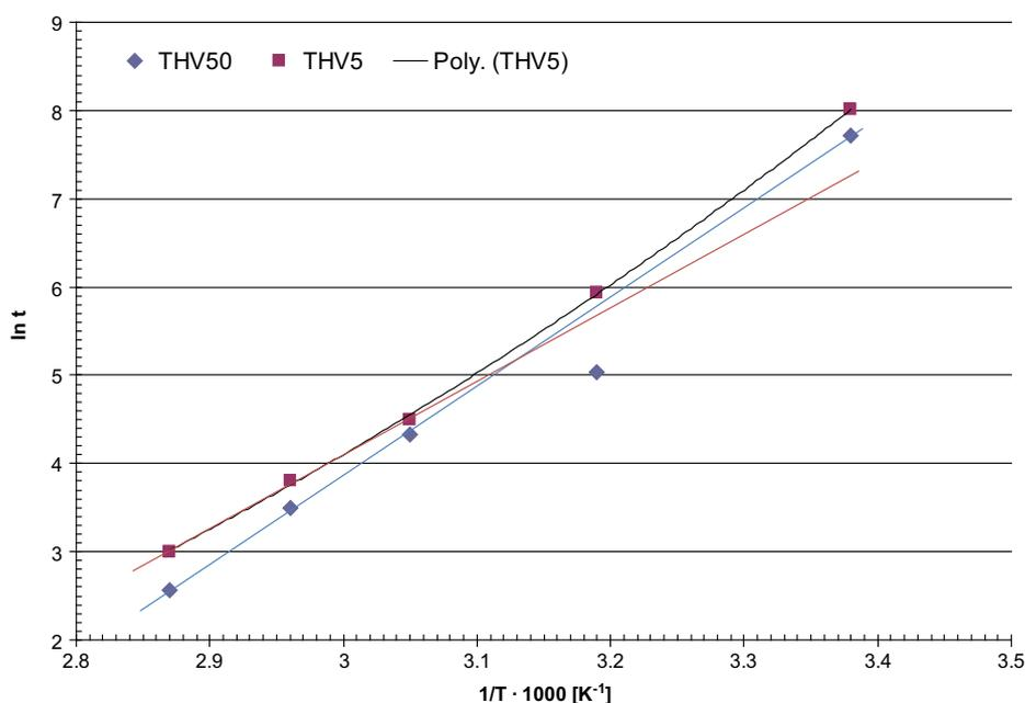
Fig. 2. Arrhenius plot using two threshold values viz. THV50 and THV5.
